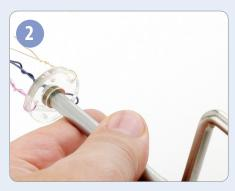
Pull the wires taut, turn the crank, and watch the wires twist.
