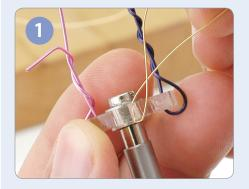
Place up to 5 Artistic Wires onto the disc of the Wire Twister, then attach the wires to a sturdy object.
