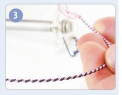
Multiple wires, once twisted, have more strength than single wires.
