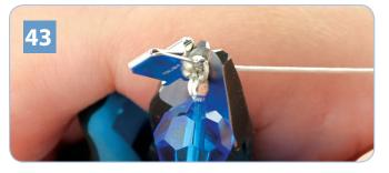
43. Cut the other remaining wire, making sure not to cut the looped wire that is holding the clasp. Note: the flush portion of the cutters is against the portion of the wire that will stay on the piece of jewelry allowing for the closest cut possible.
