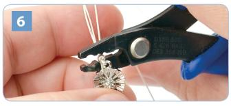
6. Carefully slide the crimp about 1/4» from the clasp, making sure the longer wire doesn't slip out of the crimp and place it in the second set of notches in the Mighty Crimping pliers as shown. Make a compression strong enough to close the jaws of the pliers as completely as possible. This should make the crimp and its contents bend into a bean shape.
