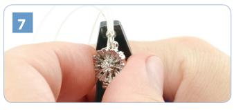
7. Carefully rotate the bean 90 degrees and place it into the front portion of the jaws of the crimping pliers. Make a compression, strong enough to close the jaws. The bean shape should fold in half to secure the wires inside. If for some reason you are not successful, you will need to cut the wire and the crimp away and begin again. It is very important that the crimp be formed then folded. This is what holds the design to the clasp.
